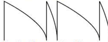
Positive Skew on a Saw Wave
